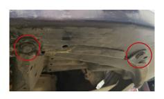
3. Remove the two push clips securing the fender liner to the bottom of the bumper.
