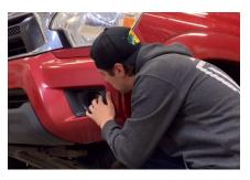
10. Loosen the 5/32" allen bolts on each side of your SS3 pod, just enough to allow you to adjust the pod.
