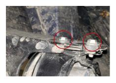
5. Pull the fender liner back and remove the two 10mm bolts holding the factory fog lamp in place. Remove the factory lamp.
