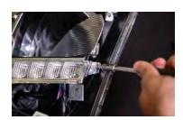
11. Reinstall the turn signal reflector by reconnecting the factory harness and reinstalling the screw that was removed in step 4.
