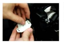
3. Using a firm grip, pull the factory board off and remove the thermal adhesion pad (sil-pad) from the back of the factory board. Reattach the sil-pad to the back of your new Diode Dynamics board.
