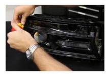
1. First, access the factory board by removing the four T-20 screws holding the black bezel in place. Once removed, pull the bezel out and set it to the side.
