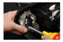
2. Next, remove the two T-20 screws holding the heatsink and black alignment bracket in place. Remove the heatsink and unclip the power connector from the factory board. Remove the two T-15 screws holding the black alignment bracket to the heatsink. Remove the final T-20 screw holding the factory board in place.
