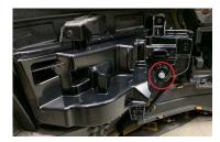
14. Test function and aim fog lamps. To do so, park 25 feet from a wall, on a flat surface. The top of the fog lamp beam pattern should be four inches lower than the height of the lamp on your vehicle. To adjust, locate the 8mm hex head bolt located on the back of the fog lamp. Rotate this bolt counter clockwise to aim downward, and counter-clockwise to aim upward. Make sure to count the number of rotations.
