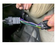
7. Unplug the factory headlight connector and install the new DRL harness provided in the kit. Then plug the harness back into the headlight. Do this on both sides of the vehicle.
