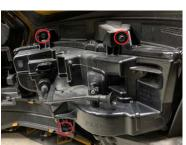
9. Remove both factory fog lamps. Using a 7mm socket, remove the three screws holding the factory fog lamps to the bumper cover and set aside.
