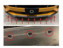
3. Using a 7mm socket, remove the fifteen lower screws holding the bumper cover to the lower splash guard.
