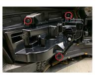
10. Install your new Elite Series combination lamps into the factory positions. Left and Right sides are displayed on the outer lens and on the backside of the housings for easy identification. Reuse the factory 7mm screws to secure the new lamps into place.
