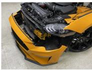
6. Remove the bumper cover. The cover will need to be lifted and rotated slightly upward to fully remove it. Disconnect the connectors from the factory fog lamps and set the cover aside.
