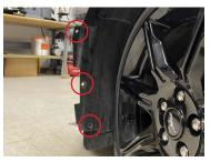
2. Using a plastic trim removal tool, remove the three push rivets holding the inner fender liner in place. Do this on both sides of the vehicle.
