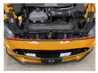
4. Using a 8mm and a 7/32" socket, remove the eight upper bolts securing the bumper cover to the core support.
