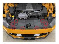
1. Using a plastic trim removal tool, remove the eight push rivets on the upper valance. Then, gently pry them off and remove the upper valance.
