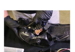
**5.** Remove the three 7mm screws holding the turn signal housing to the fog light bezel. Next, remove the turn signal housing from the bezel.
