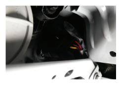
**12.** Unplug the headlight connector by depressing and pulling straight out. Plug the DRL wiring harness in line between the headlight and headlight connector.
