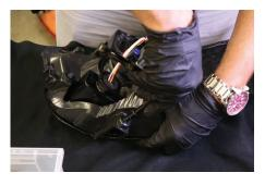
**9.** Install the new turn signal housing into the fog light bezel, reinstalling the three 7mm screws.
