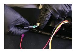
**8.** Once the blink rate has been set, insert the switch into the factory sidemarker socket. Reinstall the socket back into your new turn signal housing.
