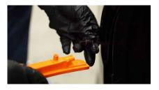
**5.** Disconnect the OEM sidemarker. Then install your new sidemarker. Test for function and secure using the two T25 torx screws.
