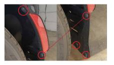
1. Remove the four push clips securing the fender liner to the bumper.
