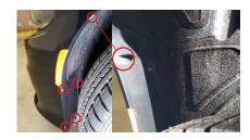
**1.** Remove five of the push clips securing the fender liner to the bumper.
